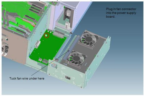
After installation of the DSP assembly and Power Supply fans is complete, re-install the power supply assembly, and internal cover in reverse order to above using the screws previously removed.
