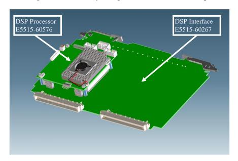
At the time of failure, the whole DSP assembly should be swapped with a new DSP which has been designed for improved reliability.
