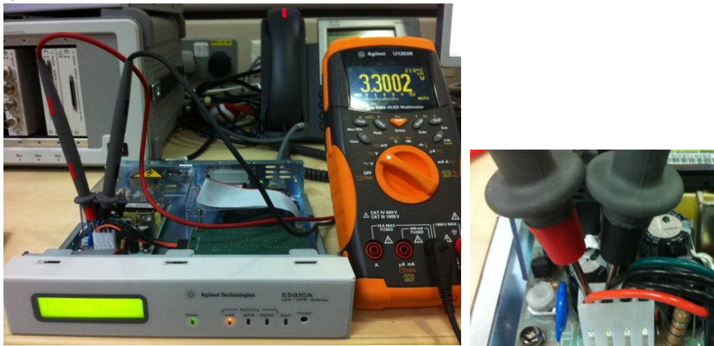
(Picture 3: Measure output Voltage with Digital Multi-meter)
