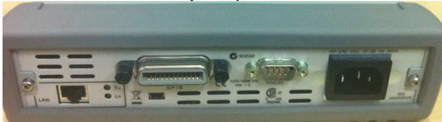
(Picture 1: Remove the Bumper attach to E5810 if any)
