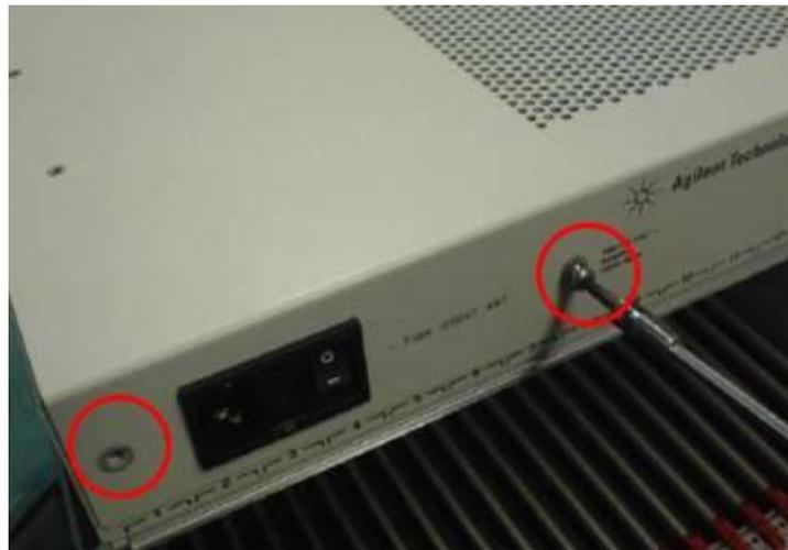
4. Unscrew the three screws (circled in red) as in the figure below.
