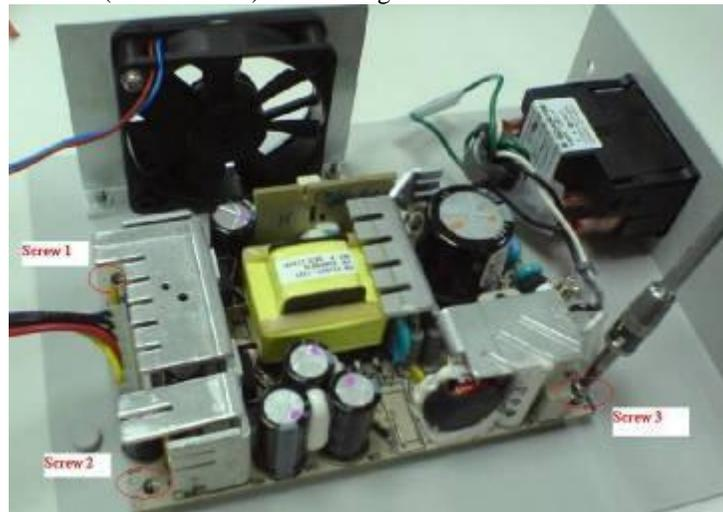
5. Check the protective cover to ensure that the grommets are present to shield the metal edges (circled in red) and the insulator sheet is to isolate the input fuse from protection cover. **Warning: Do not use the protective cover if either 'Grommet' or 'Insulator' is missing.**
