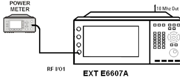
Connect the Power meter with power sensor to the **RFI/O1** output
