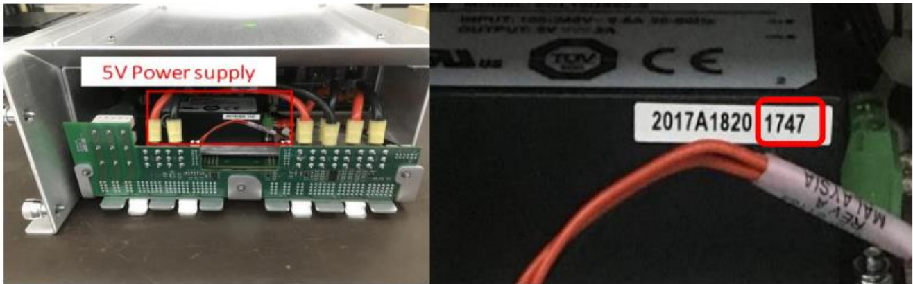
Close up view on date code ensure 1819 and above
