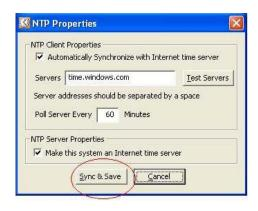
3. Open NA and connect to the Master DNA(first unit in chain) and set the Reference Clock Source to NTP. Set the IP address = to the second NIC card address (172.30.1.100 for compatibility). Leave the NA window open. Open another instance of NA Hardware Select LIM.
