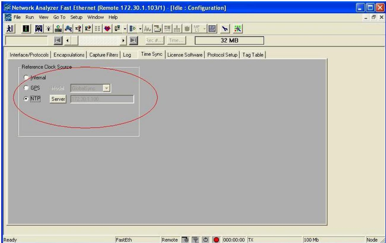
4. The Master clock in the LIM Select window should be set to NTP. Verify there are no time sync errors shown for either slave unit. Errors would be found in the Precision column.
