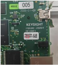
After PPMC board replace with J7201-63004 Programmed PPMC board, continue with instrument repair procedure.
