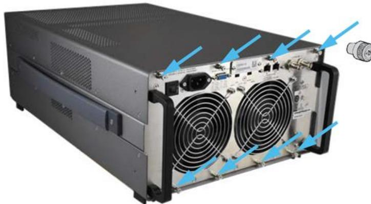
4. When all eight captive screws are loose, use the rear panel handles to pull the Rear Panel Assembly from the chassis.
