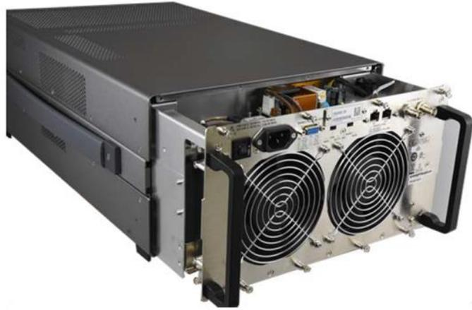
5. Carefully pull the Rear Panel Assembly all the way out of the chassis.
