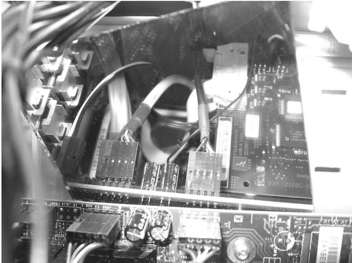
Figure 2: Results of 3.2" drop of oscilloscope (looking at mirror).
