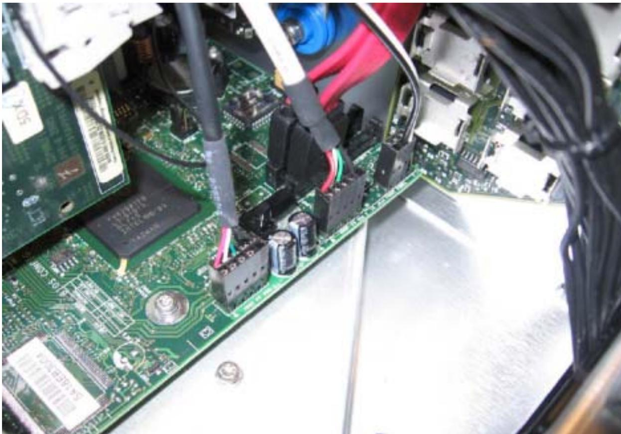
**Figure 4: Picture of cable connectors following application of RTV**
