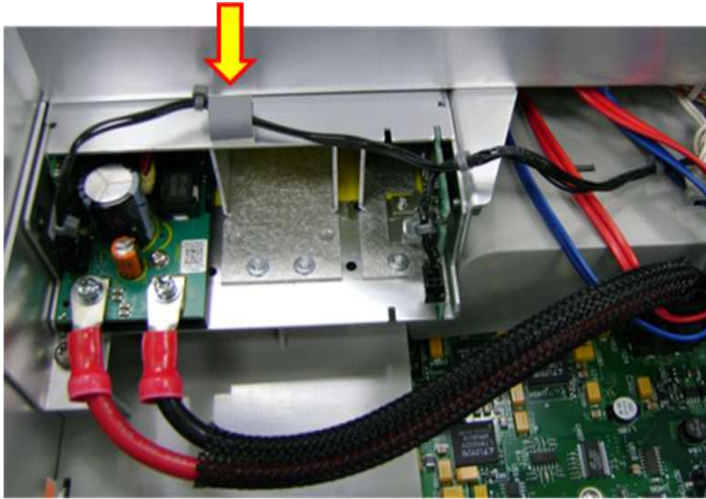
Bulk power supply cable and on/off cable routing
