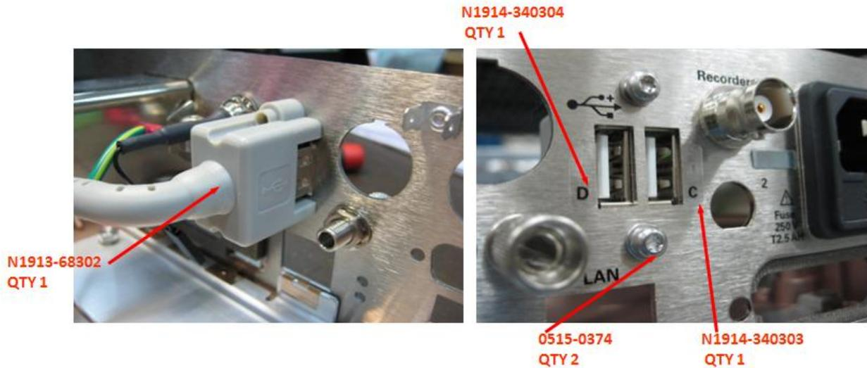
Figure 2: Connection of USB Ports to rear panel
