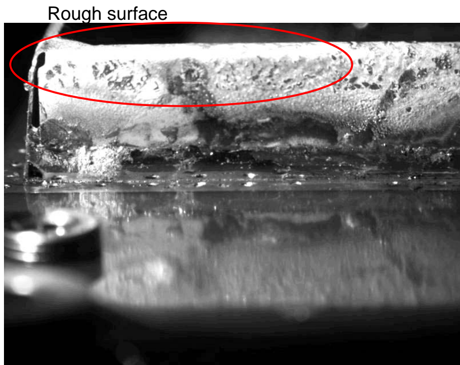
Figure 4. Ensure no excess solder wicked across the top of the shield walls. Uneven surface will prevent lid fingers to reside flat on the shields.
