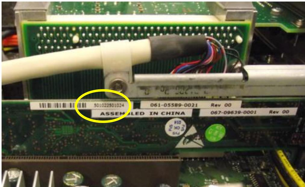
The board has a serial number (yellow circle) **NOT** starting with 200... In the case above it is: 501022501024.
