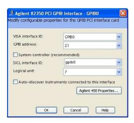
The **correct** settings shown in the picture above will make sure that the N4903B does not act as GPIB master and does not disturb communication on the GPIB bus.
