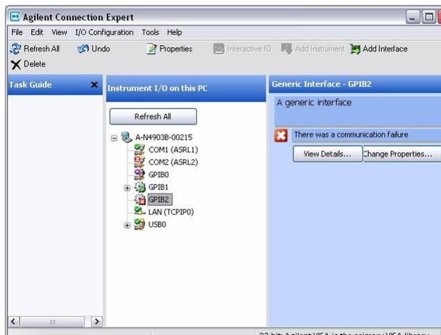
Identify the **GPIB2 interface**. It has a red cross and it shows an error in the right half of the screen. That is normal in this case. Do not get confused by that!
