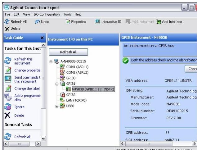
Identify the **GPIB1 interface** and notice the line underneath:
