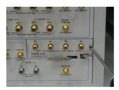
Turn on the N4903B and check whether the plug-in is recognized correctly.
