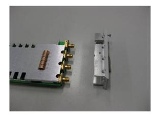
Now unscrew the lever and fasten it on the new front plate:
