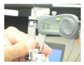
The thickness / width of the front plate should be 5.2mm (0.20in) and not 5.7mm (0.22in) as shown in the picture above.
