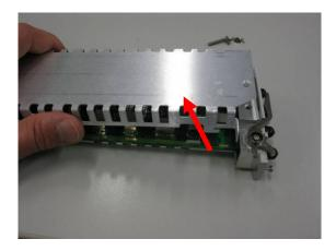
Put the cover to the side and turn the plug-in to the other side.
