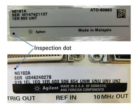
2. Check the RF assembly board serial number by pressing: *Utility > Instrument Info > Installed Board Info*
