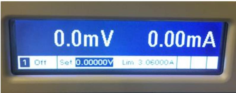
LCD (blue/white display assembly, p/n 2090-1031) has been discontinued by vendor. Replacement assembly (pictured later) is p/n 5067-6532 (amber in color). Difference in color is unfortunate, but cannot be altered.
