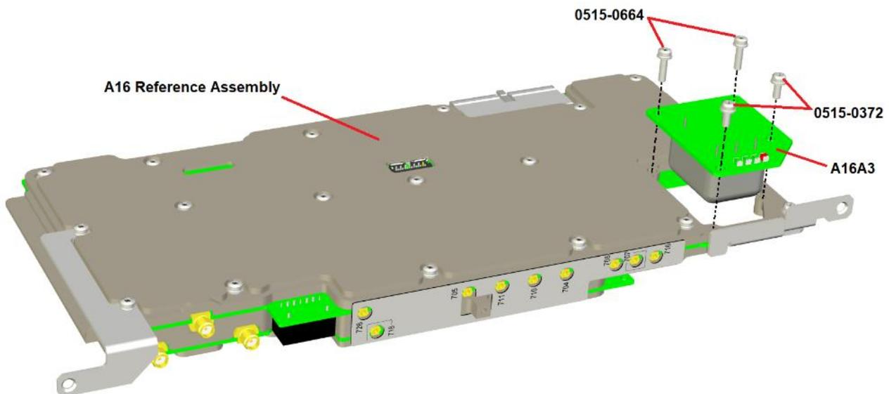
3. Install the replacement A16A3 Reference OXCO onto the A16 Reference assembly, being careful to properly plug the 26-pin interface connector in.
