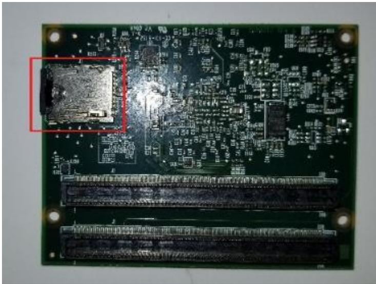
c. Using an Exacto Knife remove the Epoxy bridge holding the SD Card into the SD card socket.
