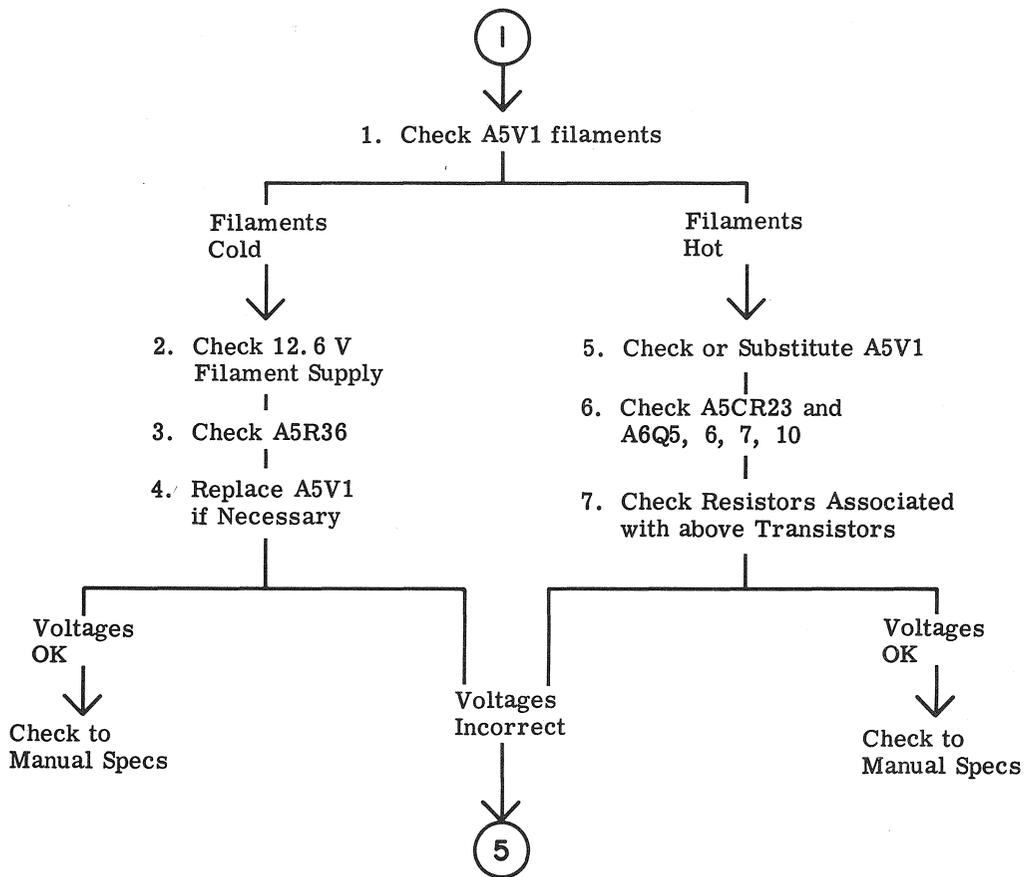
Figure 5-16. +275V and -300V Power Supply Troubleshooting Flow
