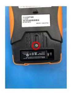
6. Loosen these 2 screws with the same Philips screwdriver.
