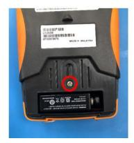
14. Install the battery cover and use a flat-head screwdriver to lock the battery cover compartment.
