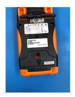
5. Loosen this screw with the same Philips screwdriver.
