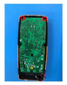
13. Install the back cover and install the screw near the battery holder.
