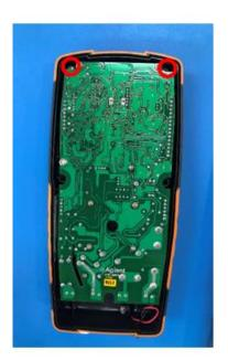
7. Gently lift the board out of the orange casing.
