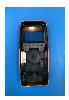
8. Loosen the 4 screws that secure the OLED display board. Then gently pull to remove the OLED display board from the PCA.
