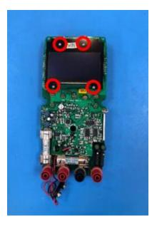
9. Next, align the new display board's connector pins with the PCA connector. Then, install the display board by pushing the connector pins into the connector on the PCA.
