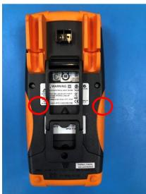
4. Lift the holder and rotate the locking mechanism to remove the battery cover with a flat-head screwdriver. Then, remove the battery cover compartment.
