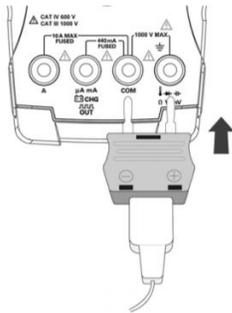
3. When a faulty temperature probe adapter is plugged in, your meter will show “OL” (open thermocouple).
