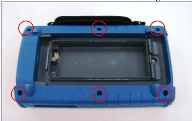
**Figure 5** Remove the screws from the rear casing
