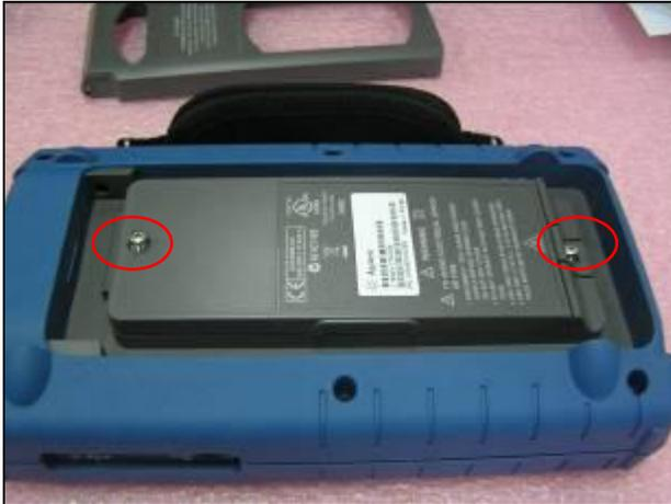
**Figure 3** Remove battery cover screws
