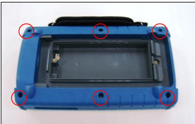
**Figure 12** Fasten the screws
