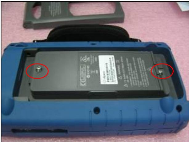
**Figure 14** Tighten the 2 screws
