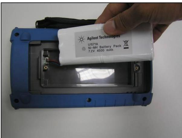
**Figure 13** Reconnect the battery
