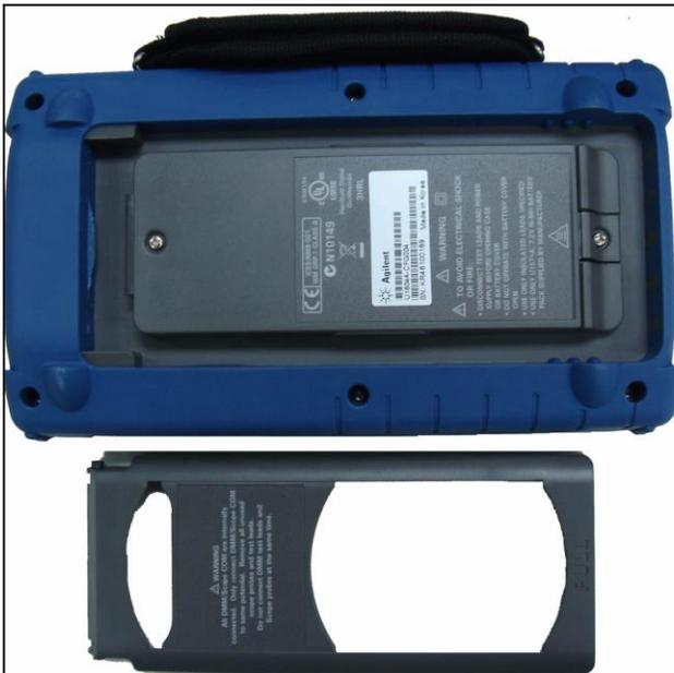
**Figure 2** Disassemble the stand from the instrument
