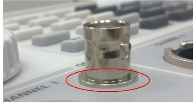
b) BNC connector securely tightened
