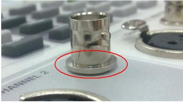
a) BNC connector not securely tightened
