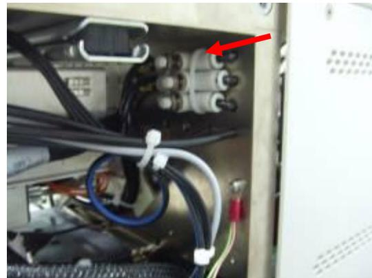
Figure 37: loosening the knob of the fittings
