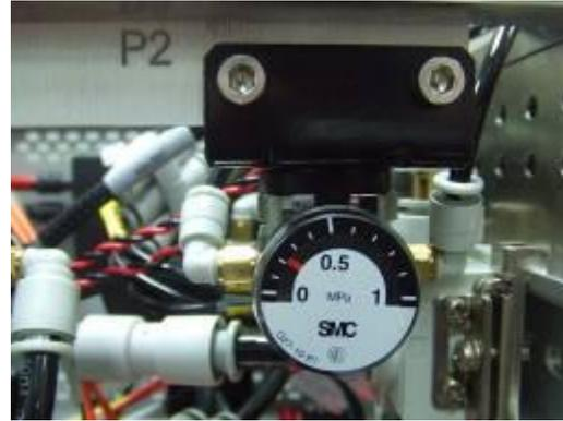
Figure 36: Pressure Regulator at P2 operating at 0.22MPa
