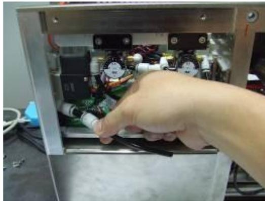
Figure 19: *Plugging the M8 tubing end from Step 16*
