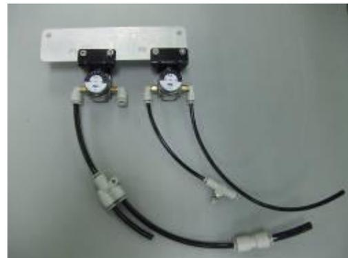
Figure 14: *Tubing and Fitting sub-assembly linked to the Pressure Regulator at P1*
