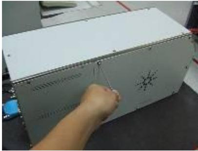
Figure 2: Dismantling Front Side Panels
