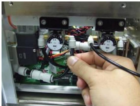
Figure 20: *Plugging the M6 tubing end*
