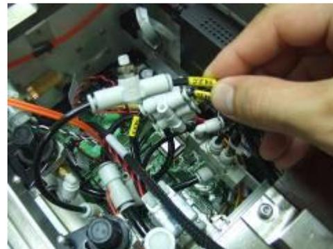
Figure 23: Plugging in the M4 tubing end
