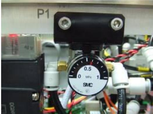
Figure 35: Pressure Regulator at P1 operating at 0.6MPa
