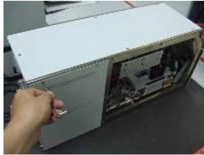
Figure 3: Dismantling Rear Side Panels
