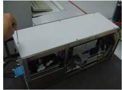
Figure 4: Dismantling Top Panel
