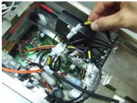
Figure 27: *Plugging in the M4 tubing end with the label of Y4.3.B into the inline flow controller B*
